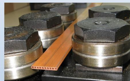
Figure 3. Copper minichannel tube being manufactured at Ohio University.
